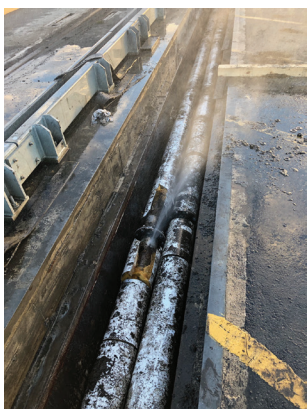
Figure 5: Corroded 316 stainless steel. Courtesy of Bulk Solutions
