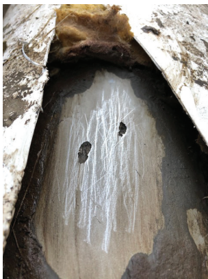
Figure 5: Corroded 316 stainless steel. Courtesy of Bulk Solutions
