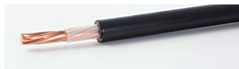
Fig. 2 — A typical CP cable construction with a PVDF barrier layer and HMWPE jacket 4 .
