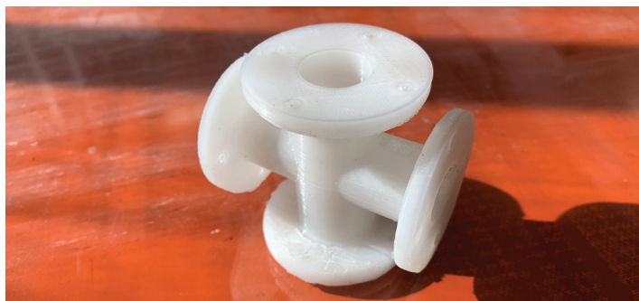
Figure 5: Complex fitting that has been 3D printed from Kynar® 826-3D PVDF filament after supports have been removed.
