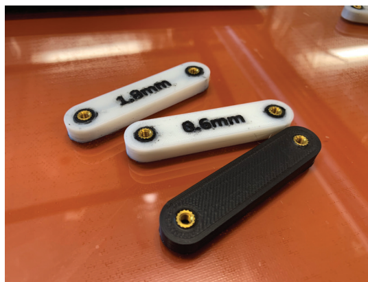
Figure 6: Three parts that have been 3D printed from PVDF resins. The white is an unfilled PVDF and the black PVDF has a conductive filler.
