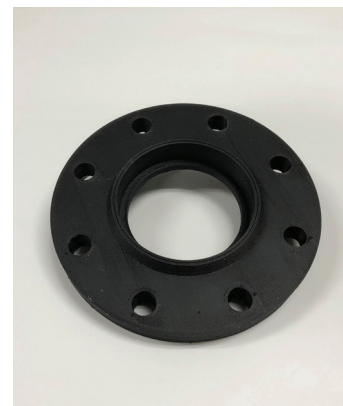
Figure 8: A large flange that has been 3D printed using PVDF filament.
