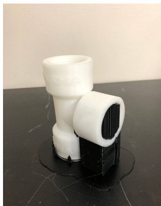
Figure 7: Support materials (black) compatible with PVDF (white), used in 3D printing a tee fitting.
