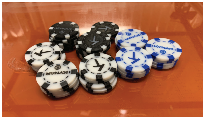
Figure 4: 3D printed poker chips, used to demonstrate multicolor and multimaterial printing with PVDF.
